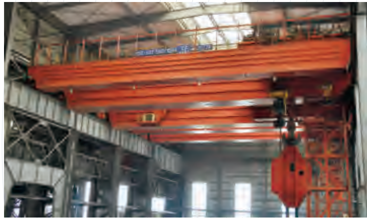
550t锻造起重机 550t Forging Crane
